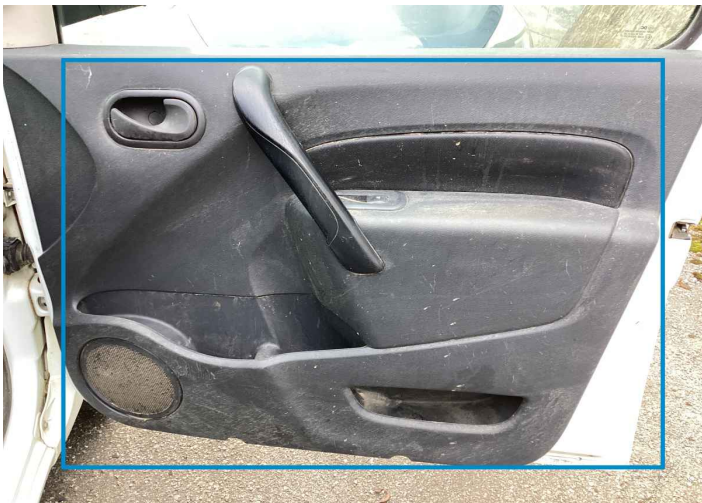
20. Panel Filling / Front Right Interior / Scraped -
