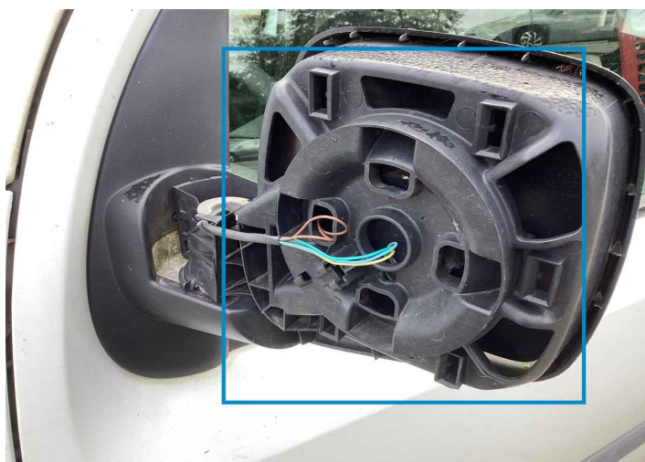
39. Mirror Shell / Front Left Missing Part -
