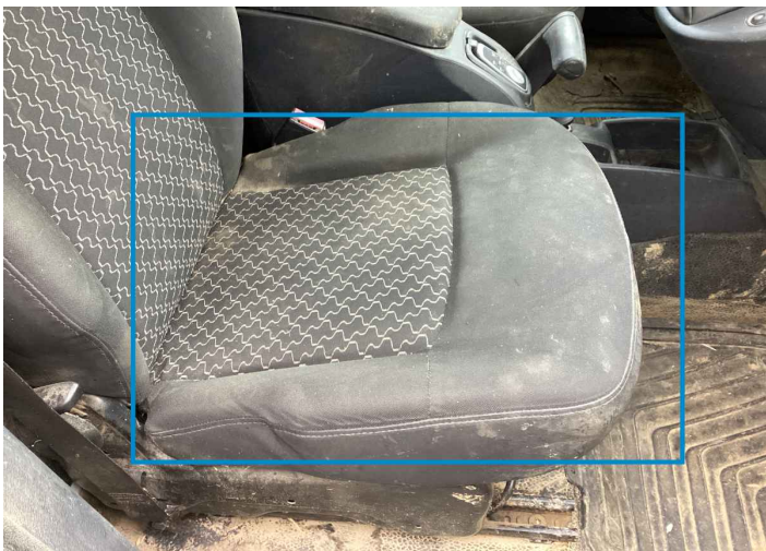
24. Seat Cushion / Front Right Interior / Stained -
