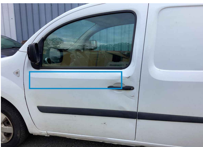
42. Door / Front Left Paint / Scratch / Line -
