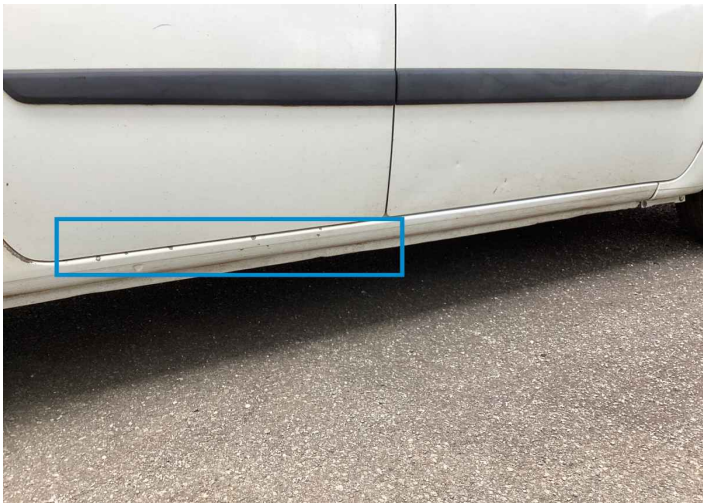
53. Rocker Panel / Center Right Paint / Chipping -
