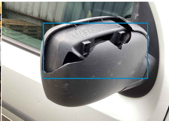
58. Mirror Shell / Front Right Bodywork / Breakage -
