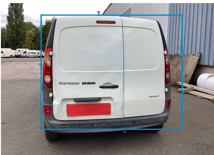
46. Tailgate Bodywork / Dent / Deformation -
