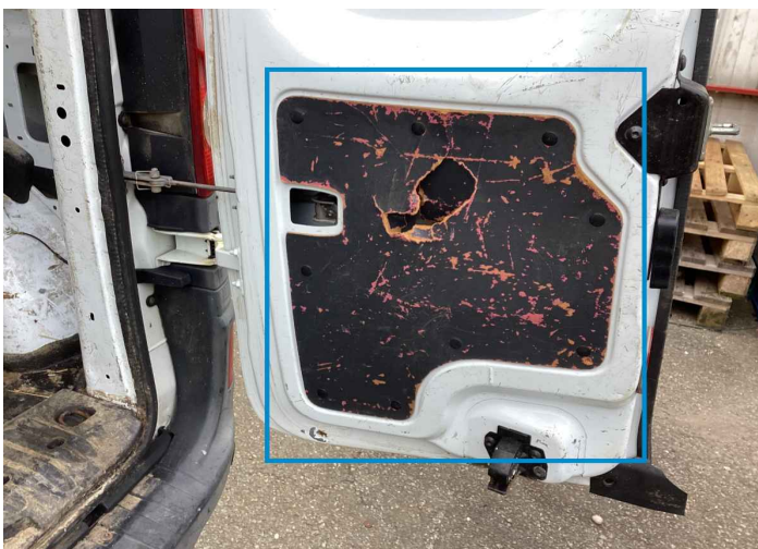
18. Trunk Upholstery / Back Interior / Broken -
