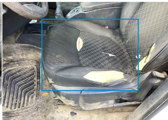
8. Seat Cushion / Front Left Interior / Stained -
