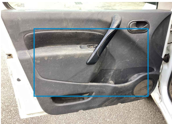
1. Panel Filling / Front Left Interior / Scraped -
