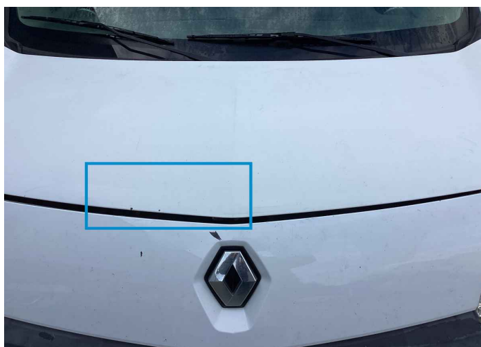
33. Hood Paint / Chipping -
