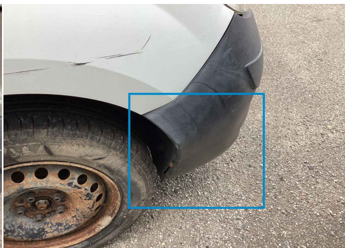
60. Corner Bumper / Front Right Bodywork / Dent / Deformation -
