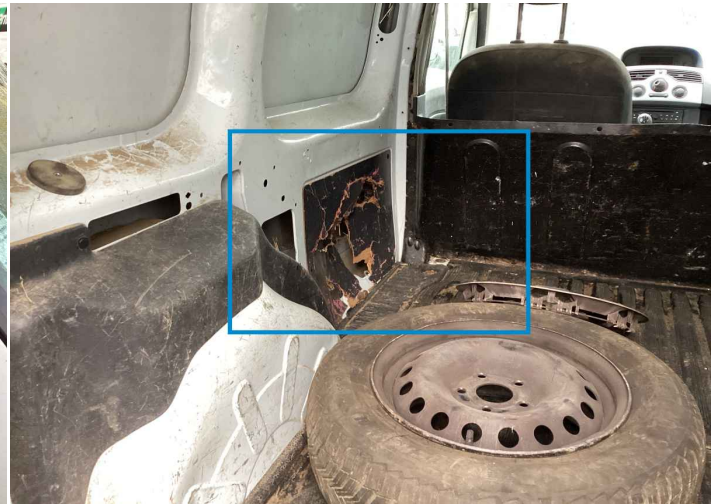
64. Trunk Upholstery / Back Interior / Broken -
