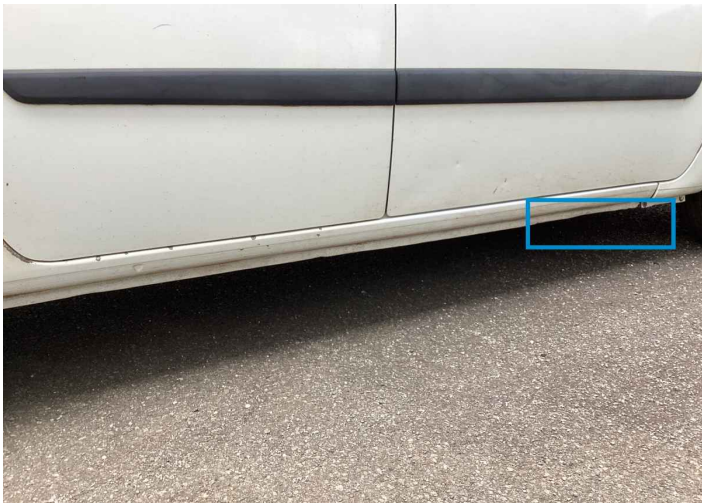
54. Rocker Panel / Center Right Bodywork / Dent / Deformation -
