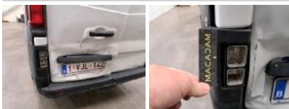
Boot door panel RL, Dent(s) and scratch(es), Replace and paint
