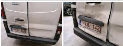
Boot door panel RR, Dent(s) and scratch(es), Replace and paint
