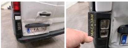
Boot door panel RL, Dent(s) and scratch(es), Replace and paint
