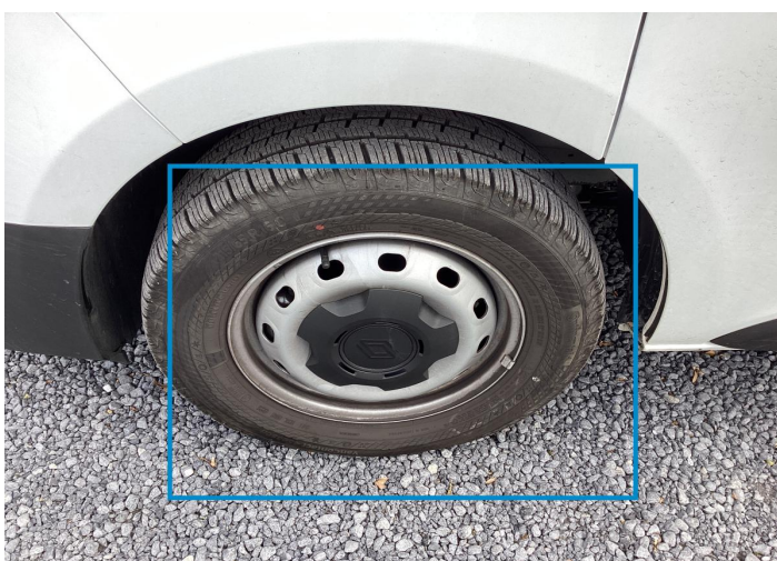
5. Rim / Front Left Out of Bodywork / Scratch -
