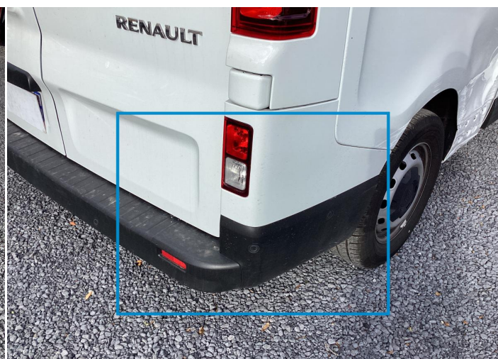
10. Corner Bumper / Back Right Paint / Scratch / Scuff -
