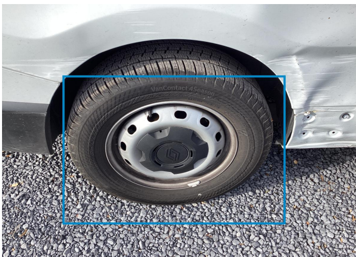
11. Rim / Back Right Out of Bodywork / Scratch -
