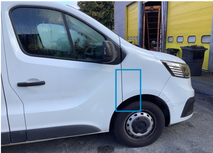
23. Fender / Front Right Bodywork / Dent / Dent -
