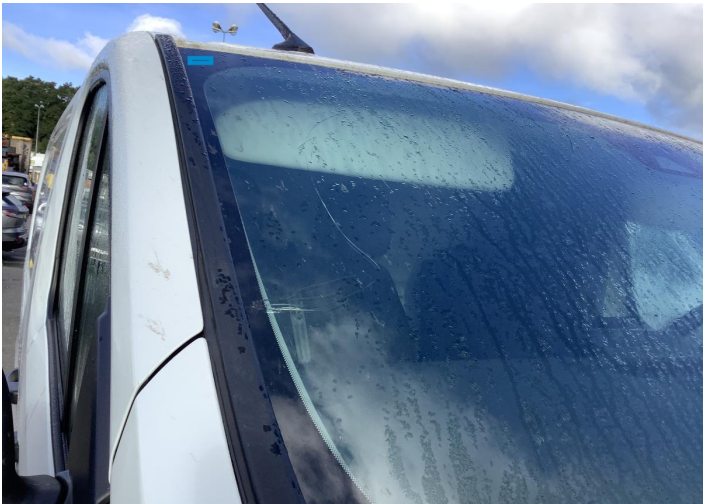
28. Windshield / Front Glass Break / Impact -
