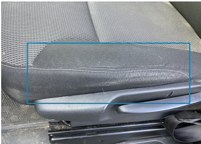
1. Seat Cushion / Front Left Interior / Worn - out -
