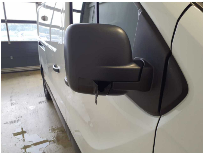
Damage 4: Wing mirror - right side: Wing mirror - Damaged - Replace
