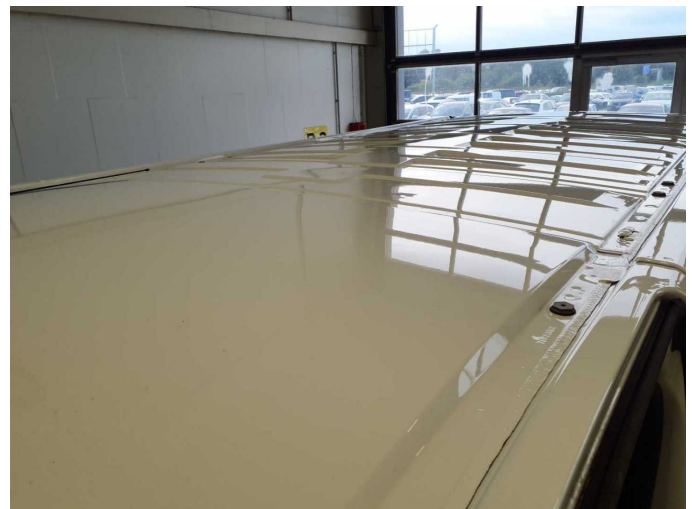
Damage 12: Roof: Roof - Deformed - Repair and paint
