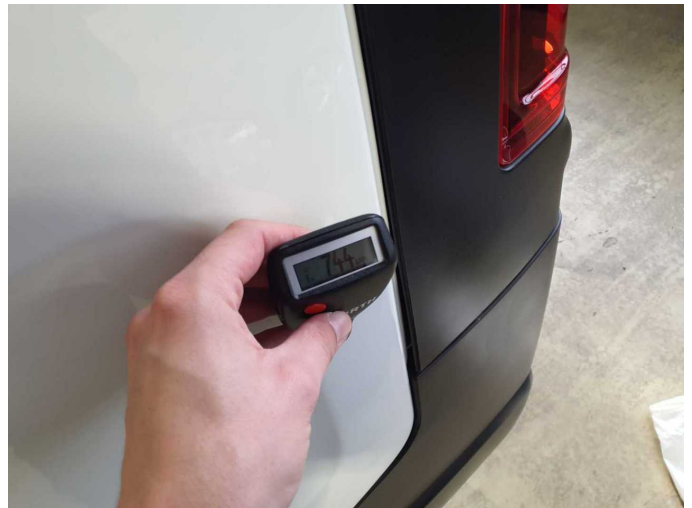
Side panel - rear left side: 744 µm
