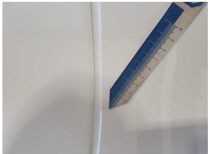
Damage 2: Side panel - rear left side: Side panel (Kleber nacharbeiten) - Unprofessionally repaired - Repair
