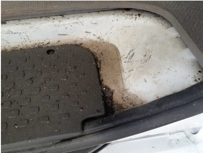
Damage 1: Body: Body - Leaking - Perform diagnosis
