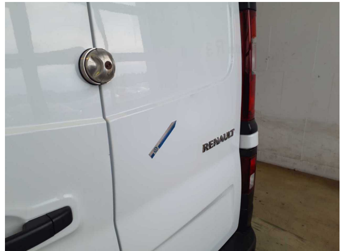
Damage 9: Boot lid / rear door: Rear door - right side - Deformed - Repair and paint
