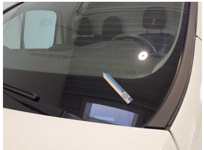
Damage 10: Vehicle glazing: Windscreen - Stone chips - Replace
