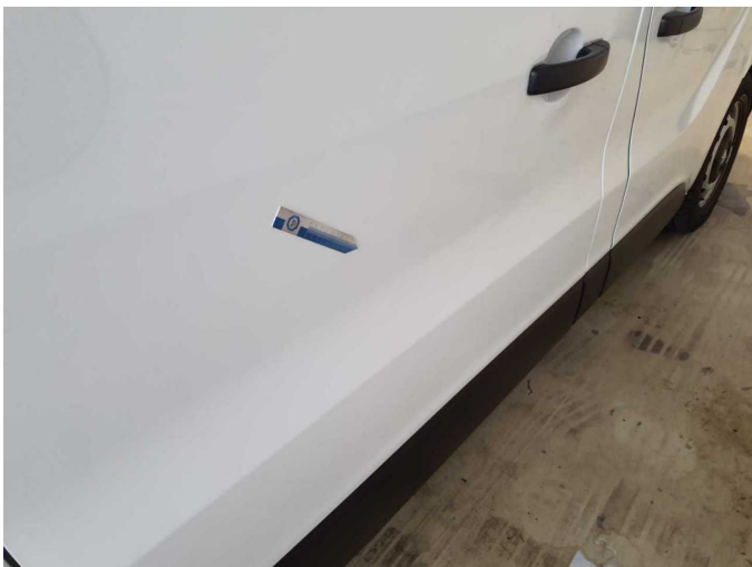
Damage 7: Sliding door, right: Sliding door - Deformed - Repair and paint
