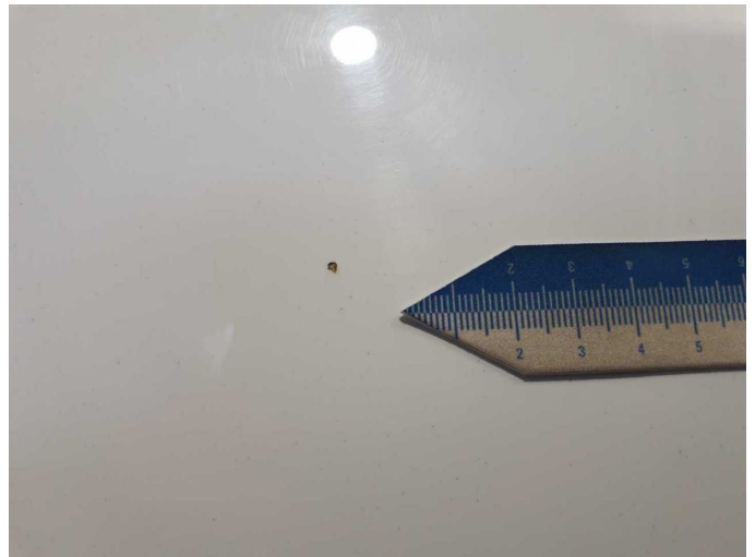
Damage 6: Bonnet: Bonnet - Corrosion - Paint
