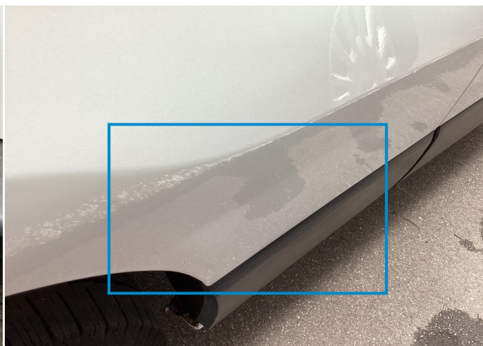
8. Side Panel / Back Right Bodywork / Dent / Deformation -
