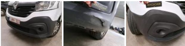
Bumper F, Scratch(es), Repair and paint (complete) 216,80
