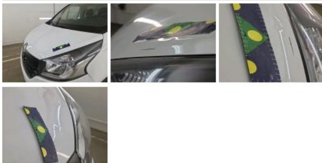
Bumper F, Crack, Replace and paint
