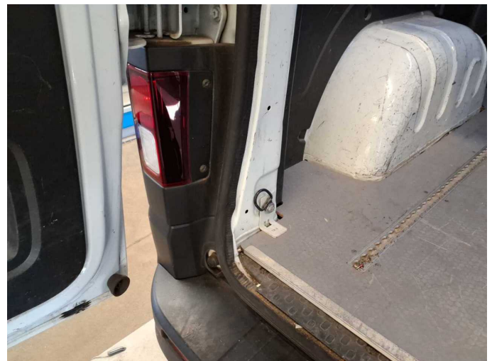
Damage 11: Boot lid / rear door: Seal - Broken / torn - Replace
