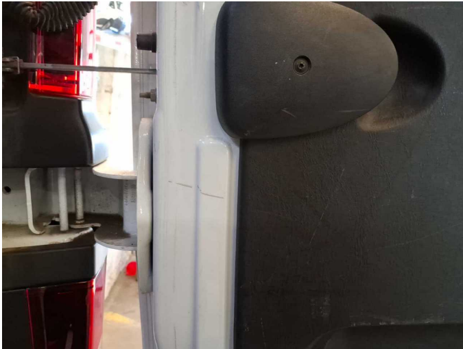
Damage 14: Interior: Cargo space division - Dent / paintcoat damage - Loss in value
