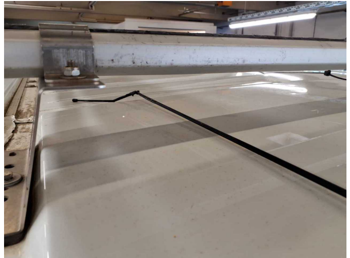
Damage 1: Roof: Stub aerial - Broken / torn - Replace
