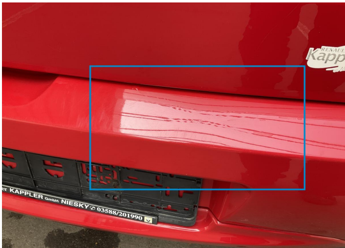
3. Bumper / Back Paint / Poor Previous Repair -
