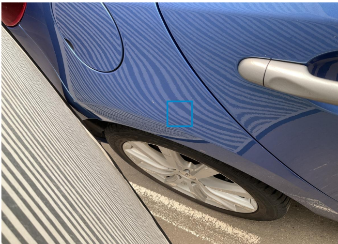
3. Side Panel / Back Right Bodywork / Dent / Dent -
