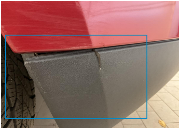
7. Bumper / Back Bodywork / Breakage / Crack -
