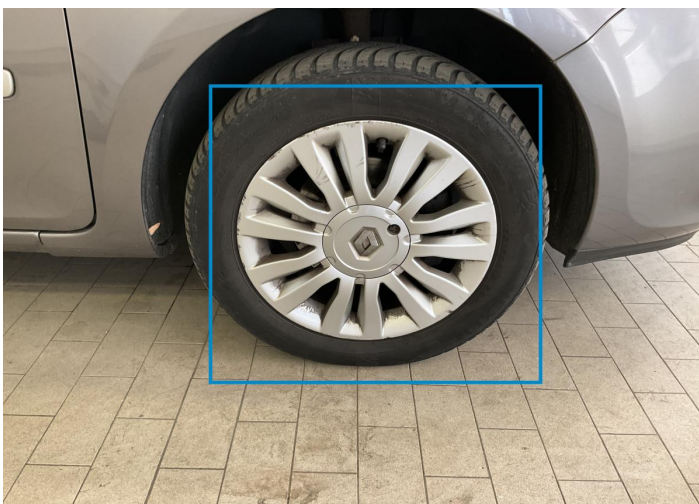
8. Rim / Front Right Out of Bodywork / Scratch -
