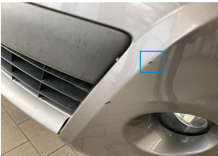
10. Bumper / Front Paint / Chipping -
