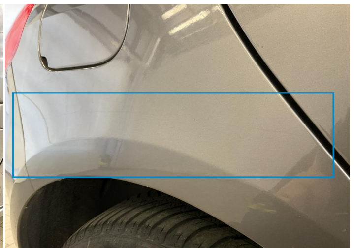
6. Side Panel / Back Right Paint / Scratch / Scuff -
