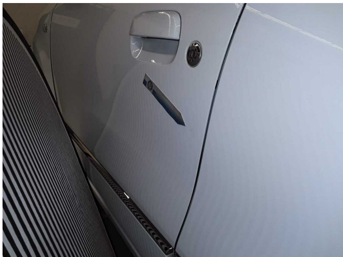
Beschädigung 4: Tür vorn links: Tür - Delle / Lackschaden - Smart Repair
