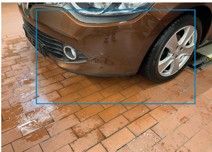
7. Bumper / Front Paint / Scratch / Scuff -
