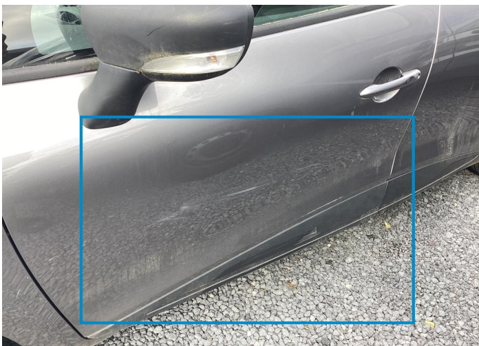
10. Door / Front Left Bodywork / Dent / Deformation -
