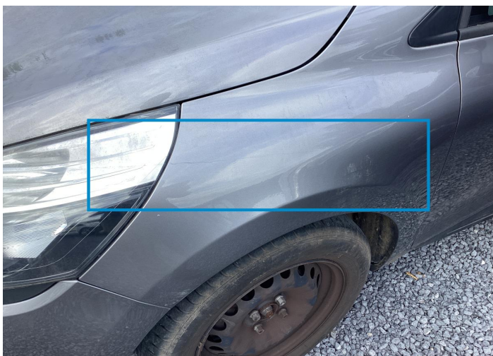
7. Fender / Front Left Paint / Scratch / Line -
