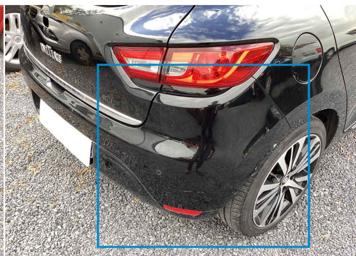
10. Corner Bumper / Back Right Paint / Scratch / Scuff -
