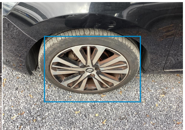
18. Rim / Front Left Out of Bodywork / Scratch -
