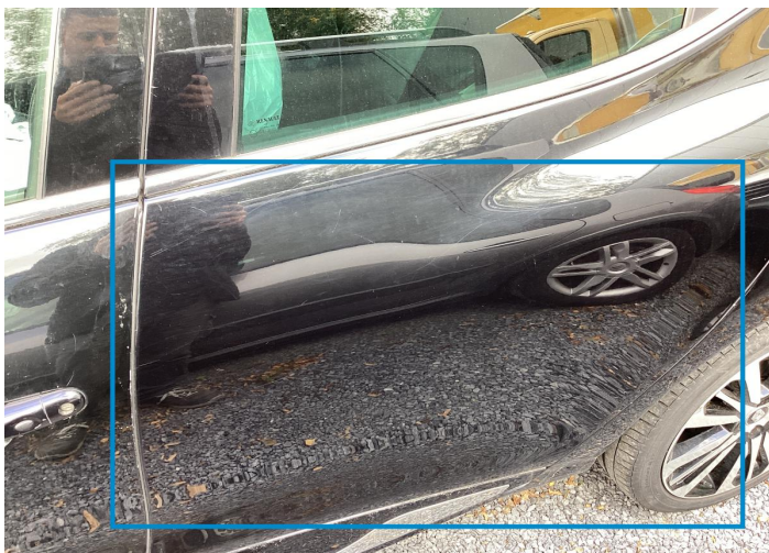
3. Door / Back Left Paint / Scratch / Line -
