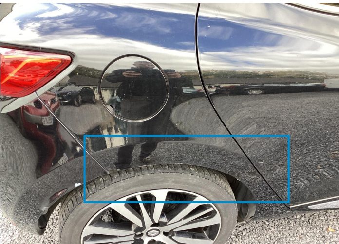
23. Side Panel / Back Right Paint / Scratch / Scuff -
