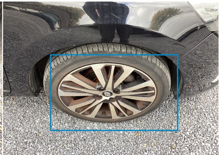
16. Rim / Front Right Out of Bodywork / Scratch -
