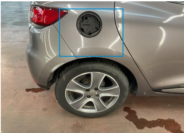
21. Fuel Door / Back Right Bodywork / Breakage -
