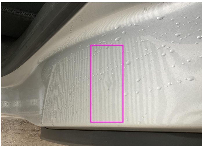
6. Rocker Panel / Center Left Bodywork / Dent / Dent -
