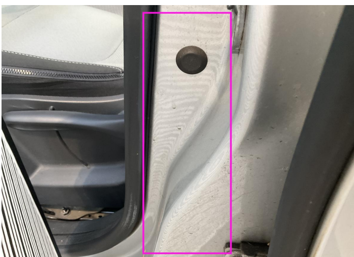
4. B Pillar / Center Left Bodywork / Dent / Dent -
