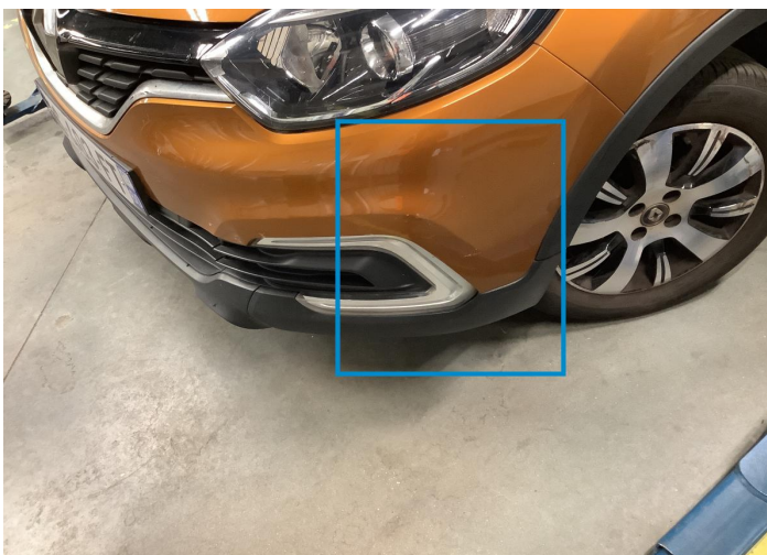
2. Shield / Front Paint / Scratch / Line -
