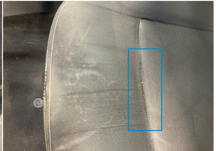
4. Seat Cushion / Front Left Interior / Ripped -
