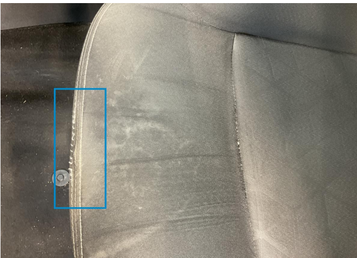
5. Seat Cushion / Front Left Interior / Ripped -
