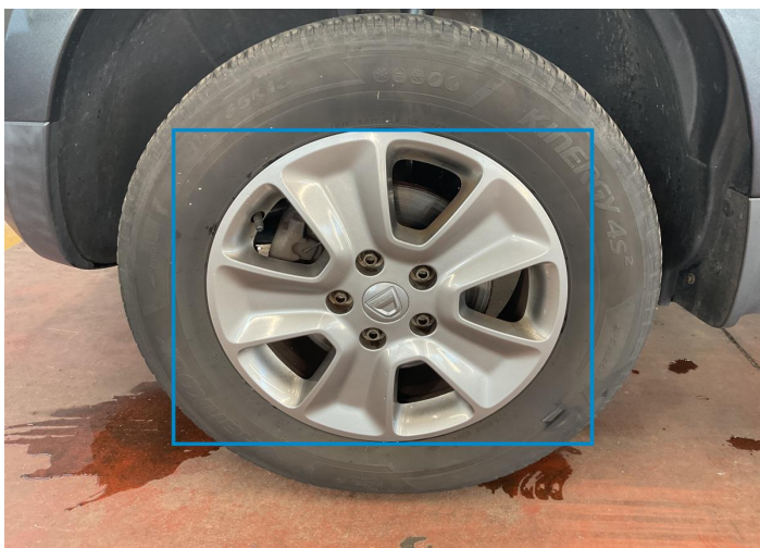
11. Rim / Front Left Out of Bodywork / Scratch -
