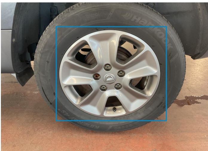
18. Rim / Back Left Out of Bodywork / Scratch -
