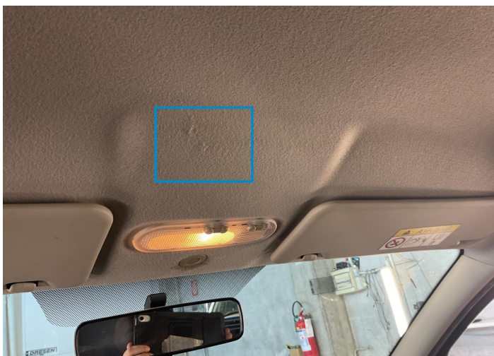
29. Roof Upholstery Interior / Ripped -
