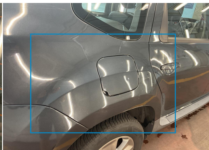
22. Fender / Back Right Bodywork / Dent -
