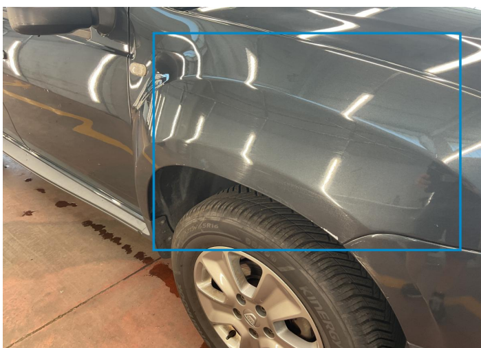
27. Fender / Front Right Bodywork / Dent -
