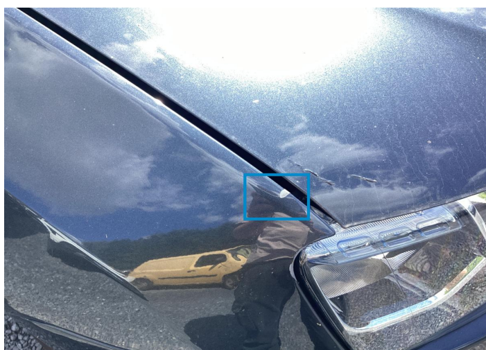
23. Fender / Front Right Paint / Chipping -
