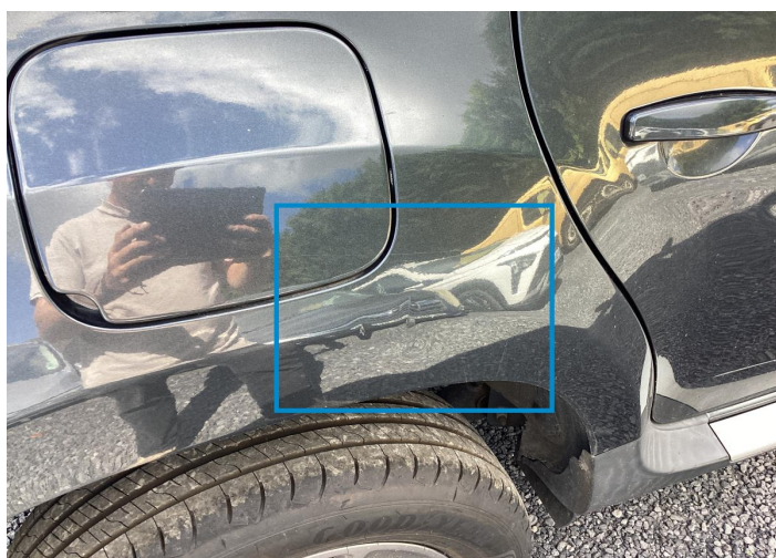
19. Side Panel / Back Right Bodywork / Dent / Deformation -
