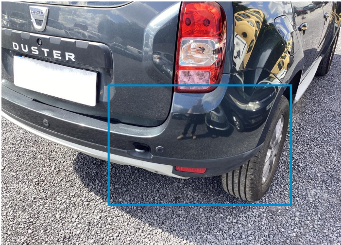
16. Corner Bumper / Back Right Paint / Scratch / Scuff -
