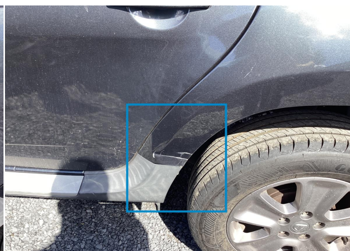
12. Side Panel / Back Left Bodywork / Dent / Deformation -
