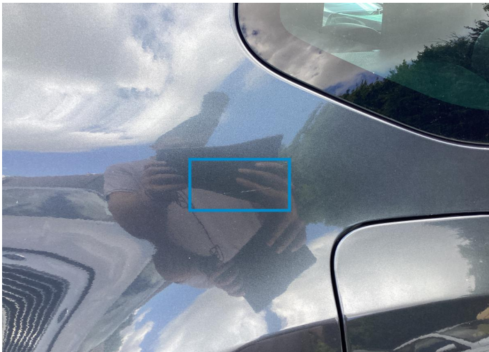
18. Side Panel / Back Right Paint / Scratch / Line -
