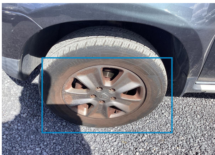
9. Rim / Front Left Out of Bodywork / Scratch -
