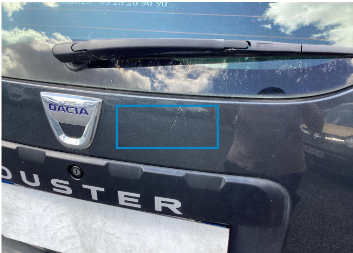
17. Tailgate Paint / Scratch / Line -
