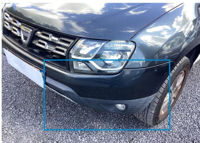
7. Corner Bumper / Front Left Paint / Scratch / Scuff -
