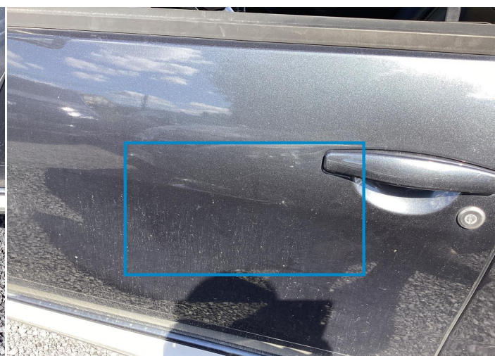
10. Door / Front Left Paint / Scratch / Line -
