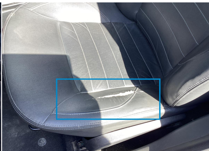
2. Seat Cushion / Front Left Interior / Holed -
