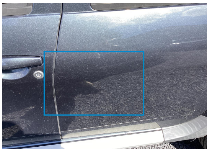
11. Door / Back Left Paint / Scratch / Line -
