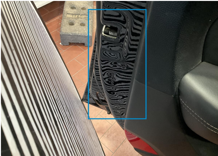
3. Door / Front Left Bodywork / Dent / Dent -
