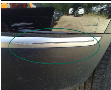
Bumper moulding / Back Right / Scratched
