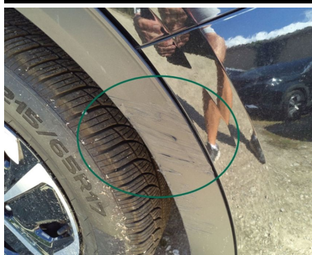
Wing moulding / Front Right / Scratched
