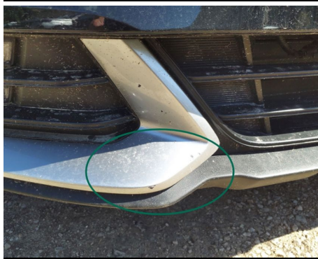
Bumper moulding / Front Right / Scratched
