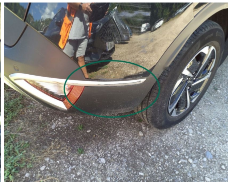
Bumper moulding / Back Right / Scratched
