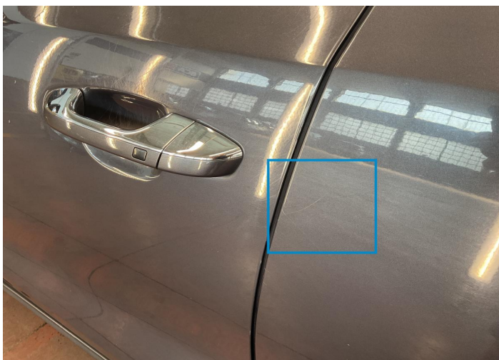
11. Door / Back Left Paint / Scratch / Line -
