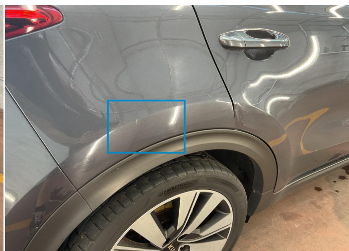
16. Fender / Back Right Bodywork / Dent -
