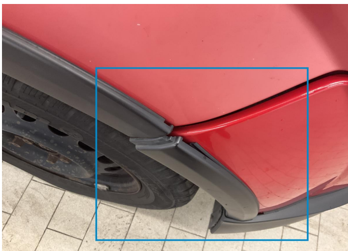
5. Bumper / Front Bodywork / Breakage / Crack -
