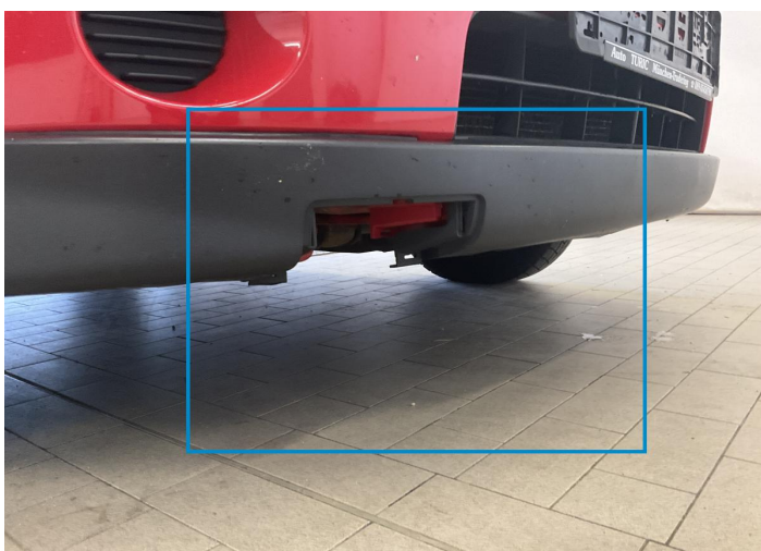
3. Shutter Cap / Front Missing Part -
