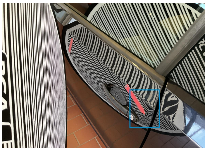
3. Door / Front Left Bodywork / Dent / Dent -
