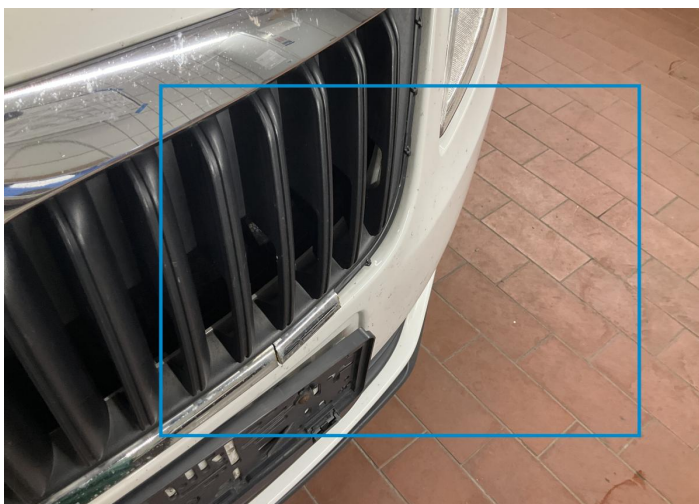
7. Grille / Front Bodywork / Breakage / Hole -
