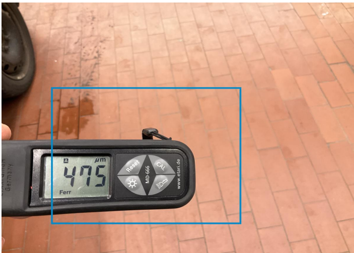
1. Door / Back Right Paint / Poor Previous Repair -
