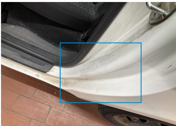
13. Pillar / Back Left Bodywork / Dent / Dent -
