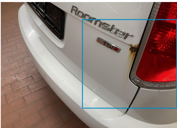
18. Tailgate Paint / Corrosion -
