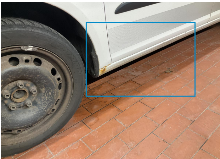
9. Rocker Panel / Center Left Paint / Corrosion -
