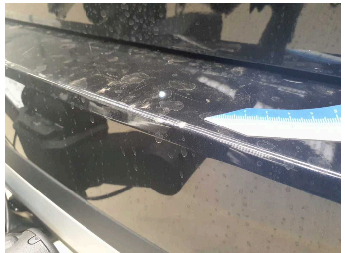
Damage 5: Rear bumper: Rear bumper (& verkratzt) - Deformed - Repair and paint
