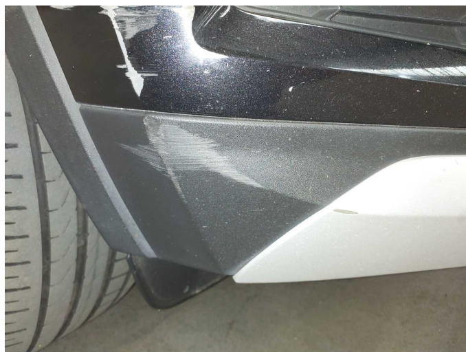
Damage 13: Front bumper: Spoiler - Scratch(es) - Smart repair
