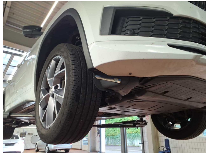
Damage 2: Body: Wheel well - front right side (Radhausschale) - Broken / torn - Replace
