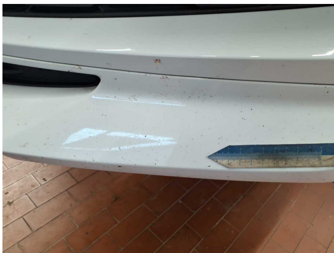
Damage 3: Front bumper: Spoiler - Stone chips - Paint
