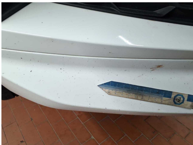
Damage 3: Front bumper: Spoiler - Stone chips - Paint
