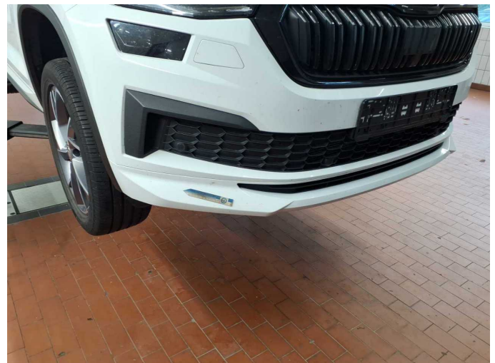
Damage 3: Front bumper: Spoiler - Stone chips - Paint
