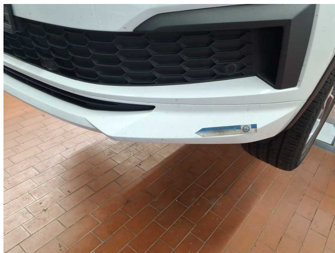
Damage 3: Front bumper: Spoiler - Stone chips - Paint
