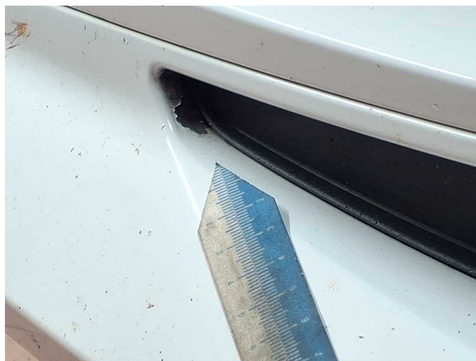
Damage 3: Front bumper: Spoiler - Stone chips - Paint
