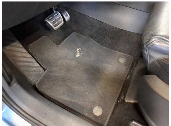
Damage 2: Trim / covers: Floor mats - Holes - Replace
