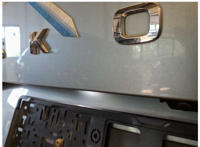
Wear and tear 8: Boot lid / rear door: Boot lid - Scratch(es) - No deduction
