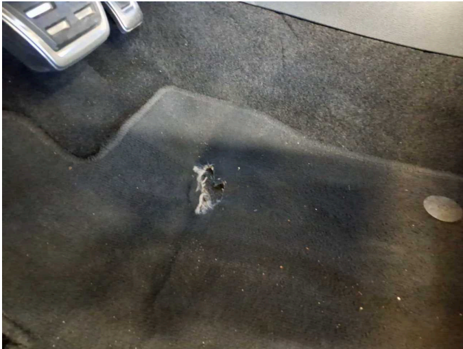
Damage 2: Trim / covers: Floor mats - Holes - Replace
