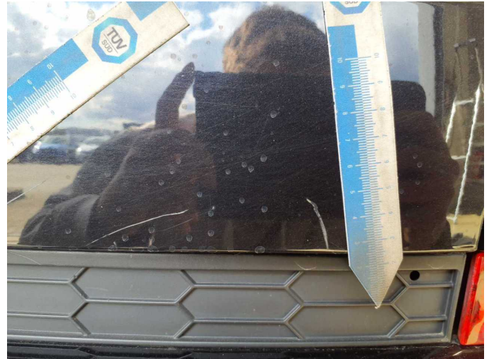
Damage 7: Boot lid / rear door: Boot lid - Scratch(es) - Smart repair
