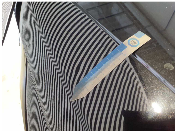
Damage 3: Bonnet: Bonnet - dent(s) - Smooth repair work
