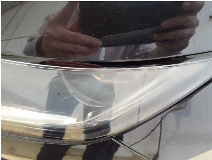
Damage 11: Headlight: Headlight - left side (Milchig) - Damaged - Replace
