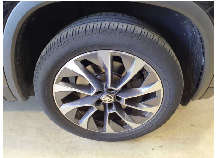
Damage 9: Wheel / tyres: Tyre - front right side - Porous / cracked - Replace
