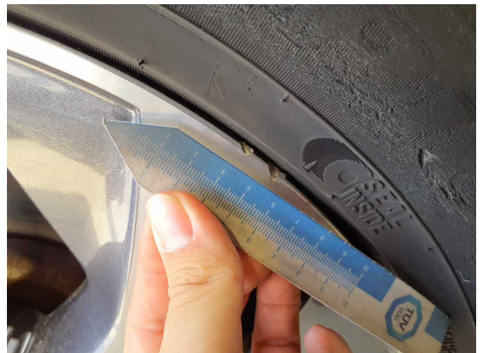
Damage 10: Wheel / tyres: Alloy rim - rear right side (Materialabtrag) - Scratch(es) - Replace
