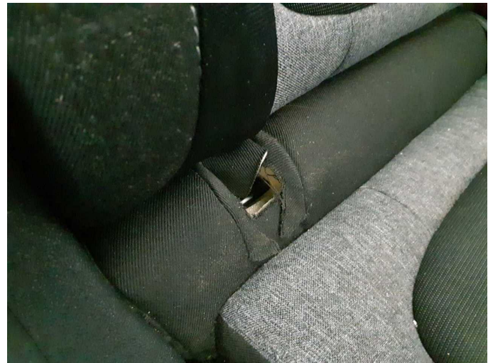
Damage 1: Seat - rear: Back seat (Isofix Abdeckung) - Missing - Replace
