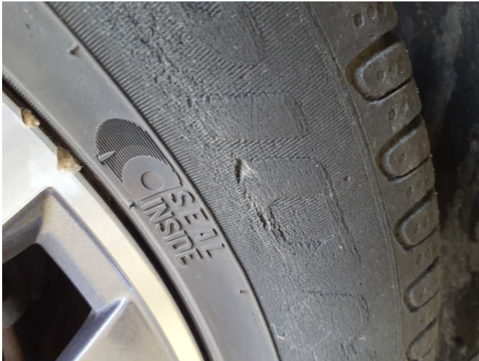
Damage 8: Wheel / tyres: Tyre - rear right side - Porous / cracked - Replace
