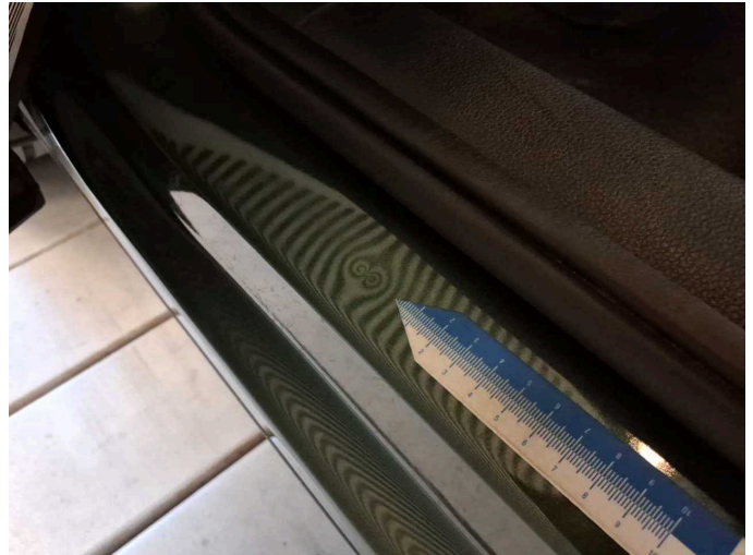
Damage 3: Sill - left side: Sill - dent(s) - Smart repair
