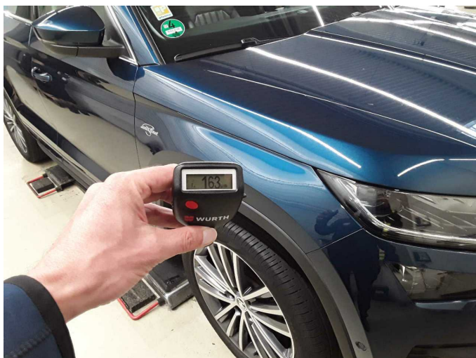
Mudguard - right side: 163 \mu m
