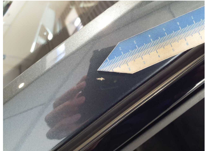
Damage 5: Body: A-pillar - left side - Stone chips - Paint
