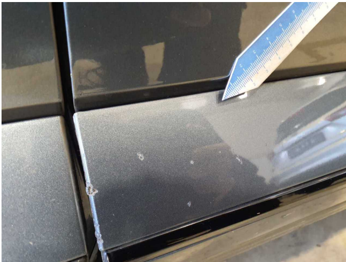
Damage 1: Door - front right side: Brightware - lower - Scratched - Paint
