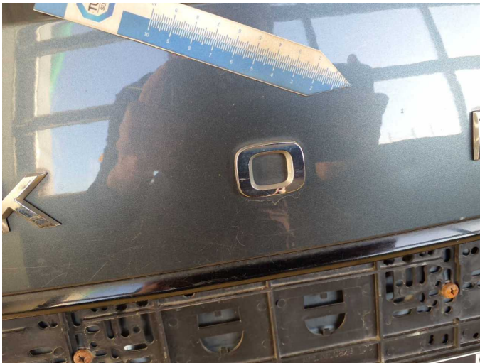
Damage 11: Boot lid / rear door: Boot lid (+ Kratzer) - Dent / paintcoat damage - Repair and paint
