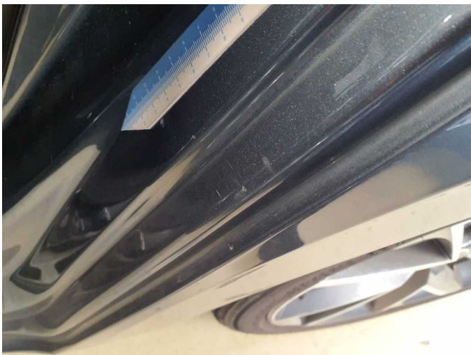
Wear and tear 5: Side panel - rear left side: Sill - Scratch(es) - No deduction
