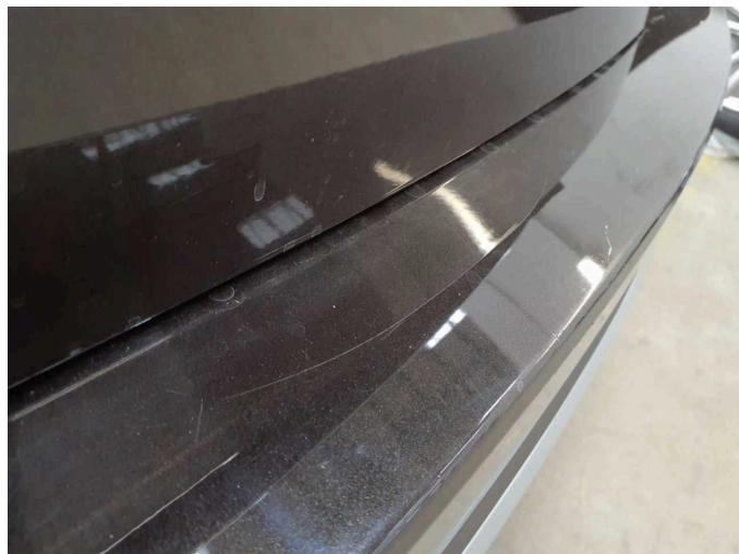
Damage 10: Rear bumper: Rear bumper - Scratch(es) - Paint
