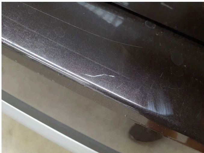
Damage 10: Rear bumper: Rear bumper - Scratch(es) - Paint
