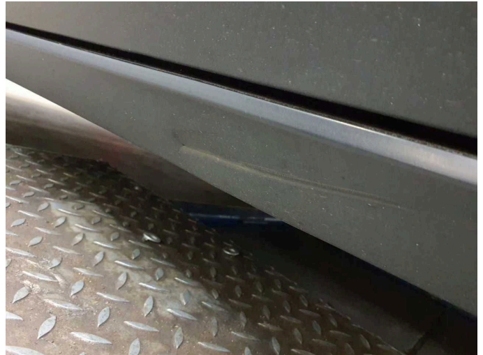
Damage 8: Sill - left side: Trim - Damaged - Replace
