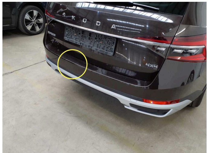
Damage 10: Rear bumper: Rear bumper - Scratch(es) - Paint
