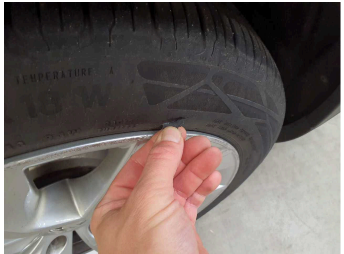
Damage 3: Wheel / tyres: Tyre - rear left side - Damaged - Replace
