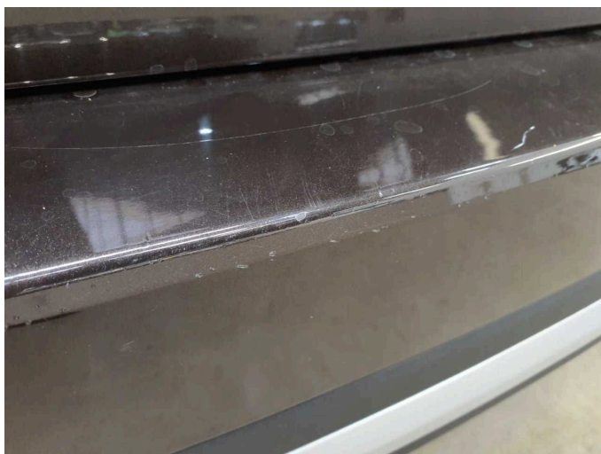
Damage 10: Rear bumper: Rear bumper - Scratch(es) - Paint
