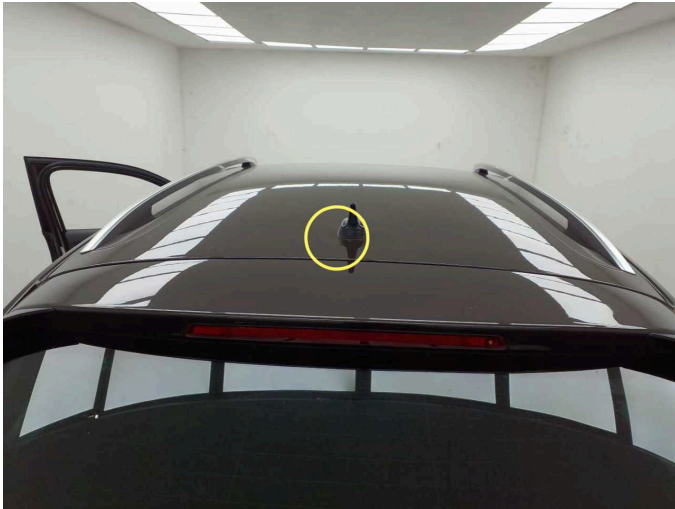
Damage 2: Roof: Roof - dent(s) - Smooth repair work
