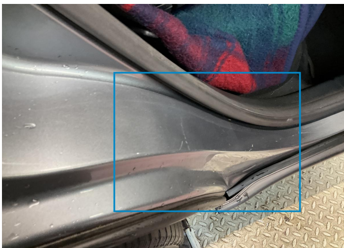
29. Pillar / Back Right Paint / Scratch / Scuff -
