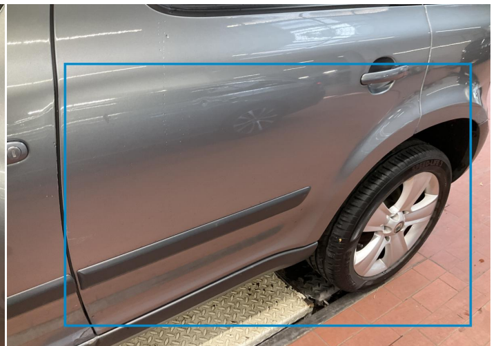
18. Door / Back Left Paint / Scratch / Scuff -
