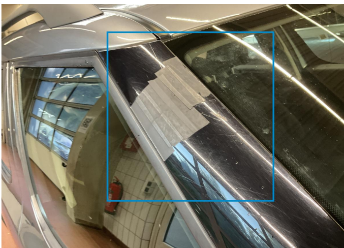
32. Pillar / Front Right Bodywork / Breakage / Hole -
