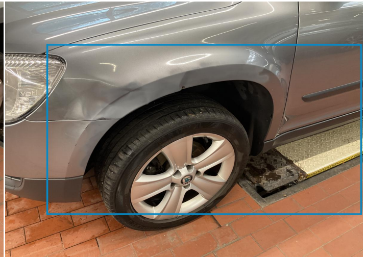
14. Wing Repeater / Left Paint / Scratch / Scuff -
