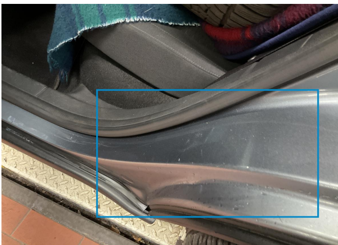
20. Pillar / Back Left Paint / Scratch / Scuff -
