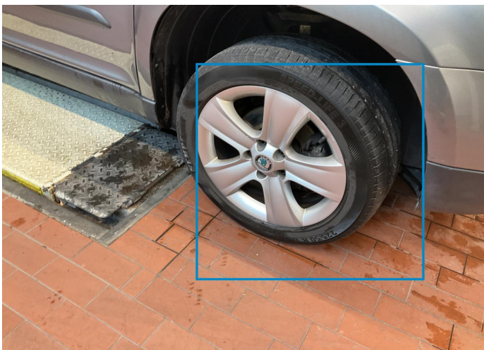
34. Rim / Front Right Out of Bodywork / Scratch -
