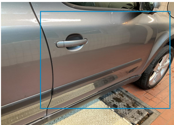
31. Door / Front Right Paint / Scratch / Scuff -
