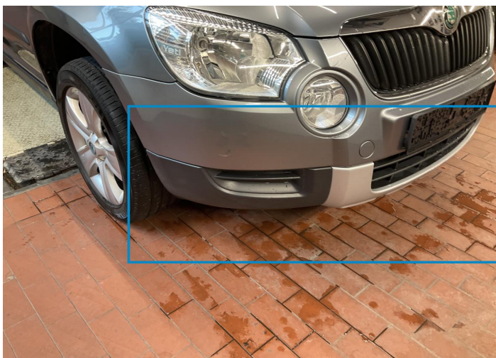
35. Bumper / Front Paint / Scratch / Scuff -
