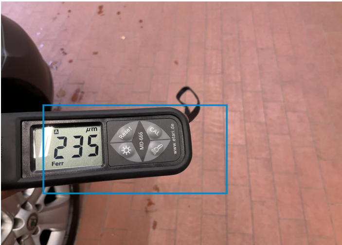
2. Door / Back Left Paint / Poor Previous Repair -
