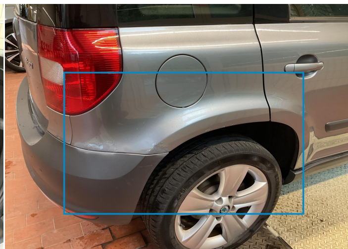
26. Side Panel / Back Right Paint / Corrosion -
