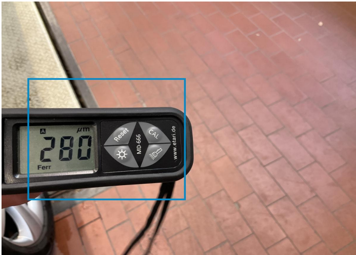
3. Tailgate Paint / Poor Previous Repair -
