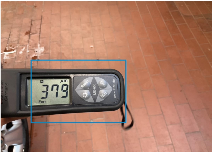
6. Door / Front Right Paint / Poor Previous Repair -
