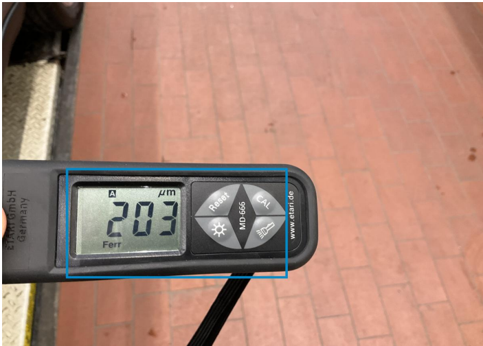
1. Door / Front Left Paint / Poor Previous Repair -
