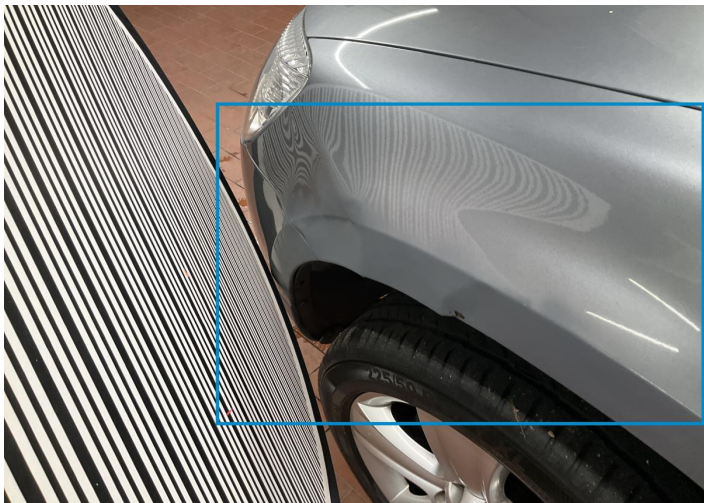
7. Wing Repeater / Left Bodywork / Dent / Dent -
