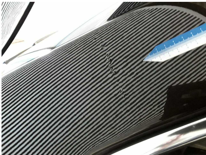
Damage 9: Side panel - rear right side: Side panel (inkl. Schaden inst.) - Unprofessionally repaired - Repair and paint
