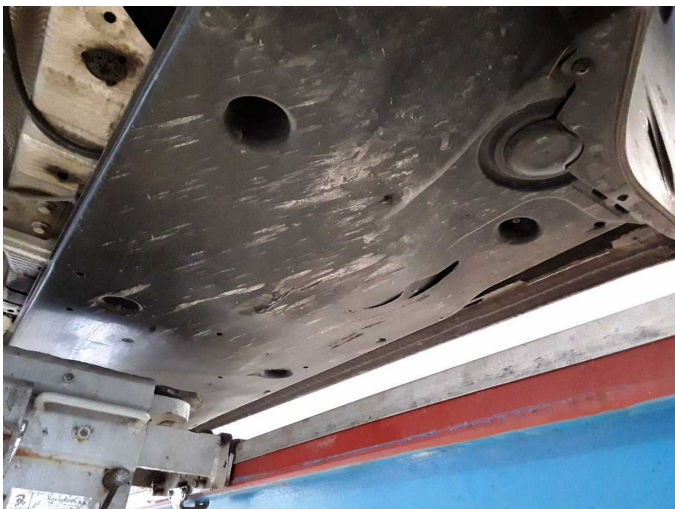
Damage 2: Body: Underbody panelling (links) - Broken / torn - Replace
