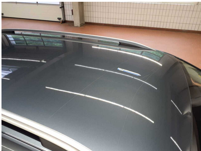
Damage 13: Roof: Roof - Scratched - Paint
