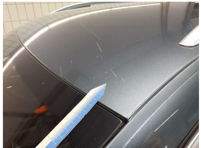
Damage 13: Roof: Roof - Scratched - Paint
