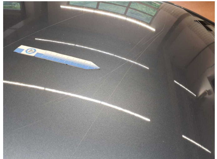
Damage 13: Roof: Roof - Scratched - Paint
