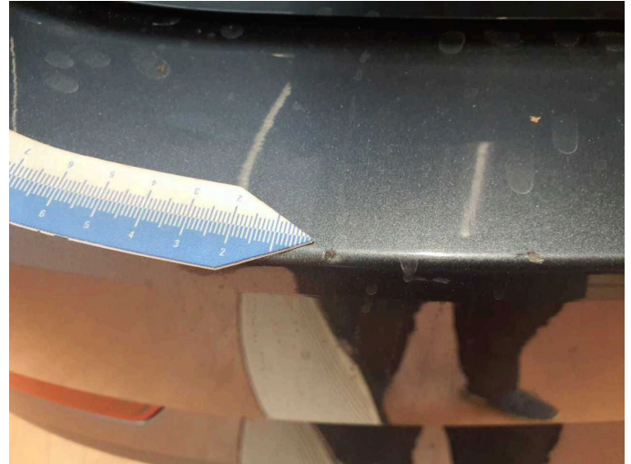
Damage 10: Rear bumper: Rear bumper - Scratched - Paint
