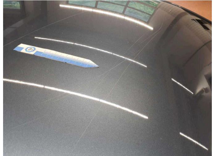
Damage 13: Roof: Roof - Scratched - Paint
