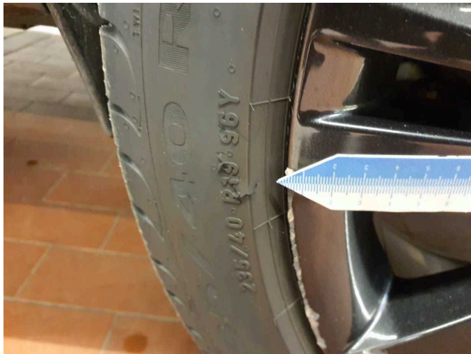
Damage 5: Wheel / tyres: Tyre - rear left side - Damaged - Replace
