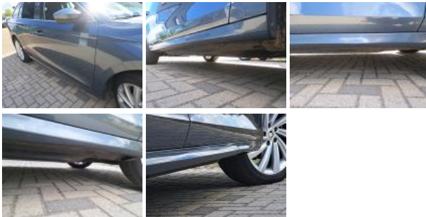
Outer sill R, Deformed / Strained, Repair and paint (complete)
