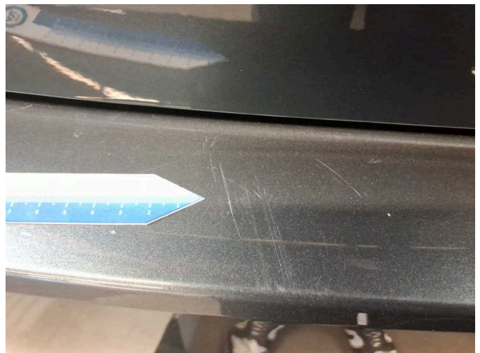
Damage 13: Rear bumper: Rear bumper - Scratch(es) - Paint
