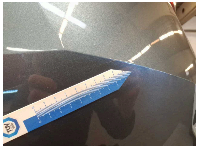
Damage 13: Rear bumper: Rear bumper - Scratch(es) - Paint
