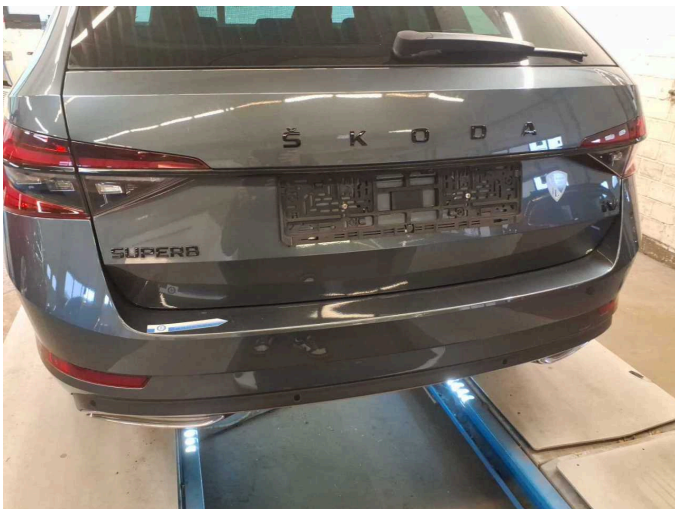
Damage 13: Rear bumper: Rear bumper - Scratch(es) - Paint
