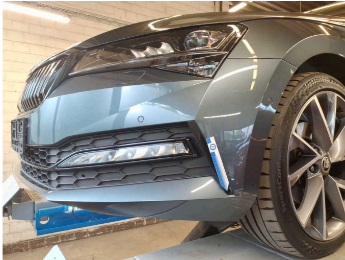
Damage 3: Trim / covers: Brightware / decorative strip - Scratch(es) - Smart repair
