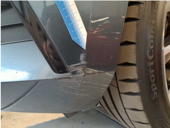
Damage 16: Front bumper: Front bumper - Scratch(es) - Paint
