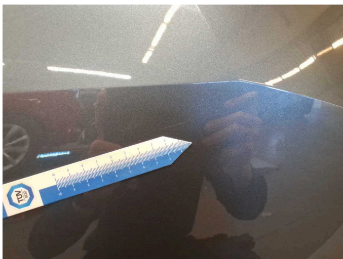
Damage 13: Rear bumper: Rear bumper - Scratch(es) - Paint
