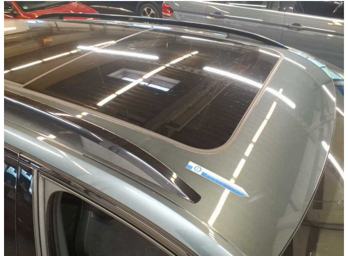
Damage 18: Roof: Roof - Scratch(es) - Paint
