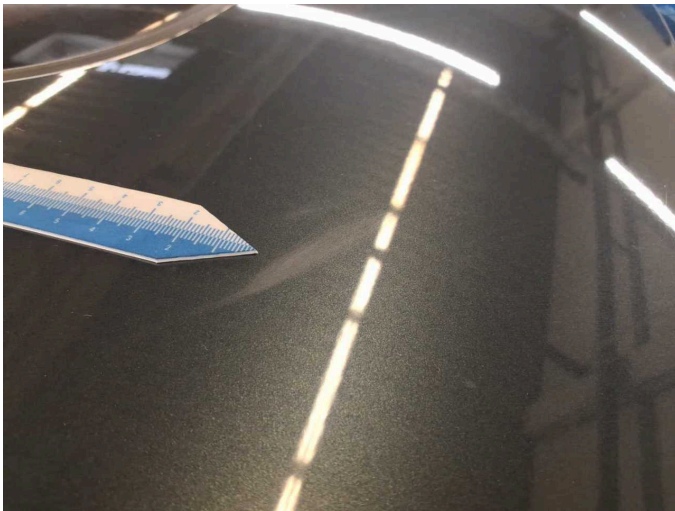
Damage 18: Roof: Roof - Scratch(es) - Paint
