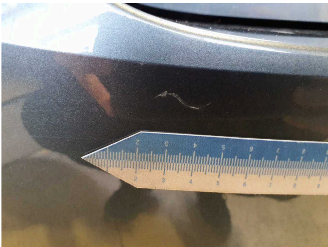
Damage 12: Rear bumper: Rear bumper - Scratch(es) - Paint
