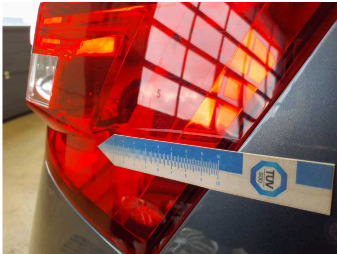
Damage 3: Tail light: Tail lamp - right side - Scratch(es) - Loss in value
