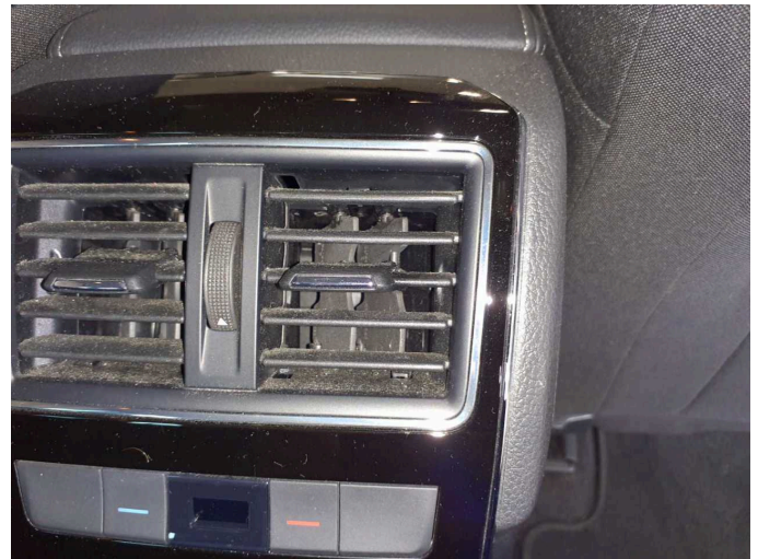
Damage 9: Instrument panel: Air nozzle - centre (Hinten) - Damaged - Replace
