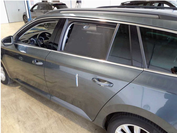
Damage 8: Door - rear left side: Door - Scratch(es) - Smart repair
