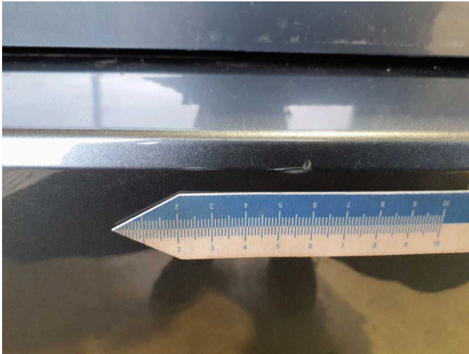
Damage 12: Rear bumper: Rear bumper - Scratch(es) - Paint
