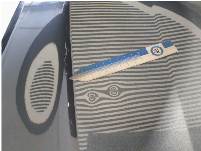
Damage 5: Bonnet: Bonnet - dent(s) - Smart repair
