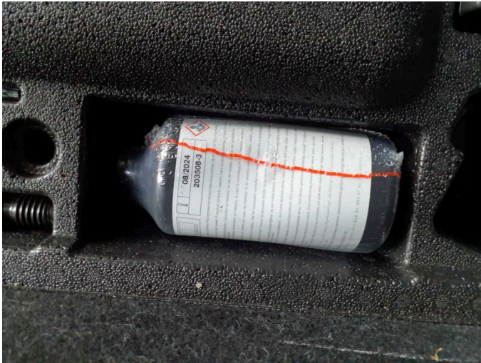
Damage 1: Equipment: Tirefit filler - Expired - Replace
