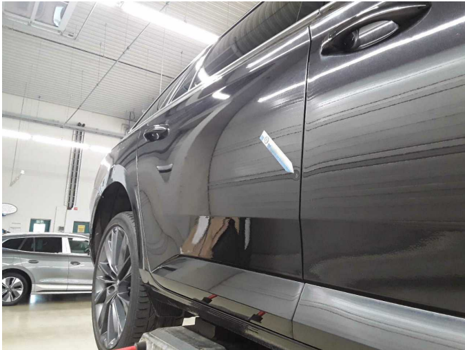
Damage 6: Door - rear right side: Door - dent(s) - Smart repair
