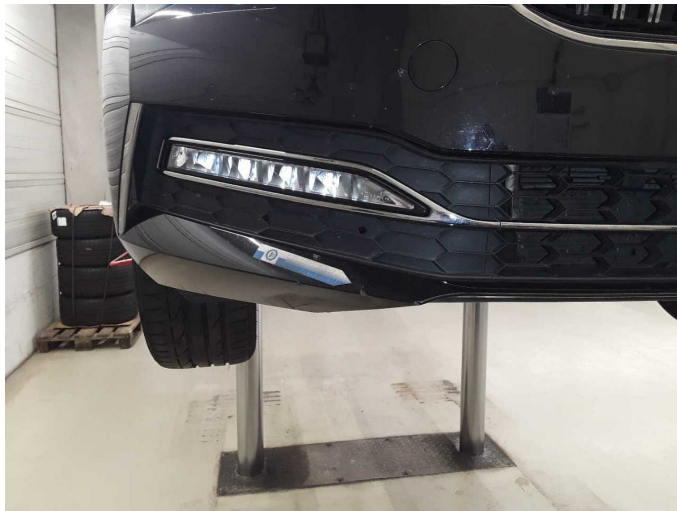
Damage 9: Front bumper: Front bumper - Scratched - Paint
