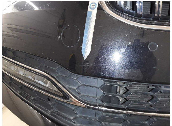
Damage 9: Front bumper: Front bumper - Scratched - Paint
