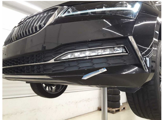
Damage 9: Front bumper: Front bumper - Scratched - Paint
