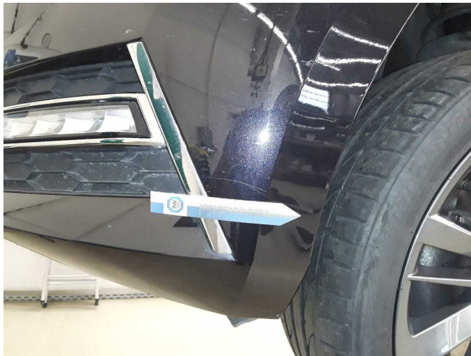
Damage 9: Front bumper: Front bumper - Scratched - Paint
