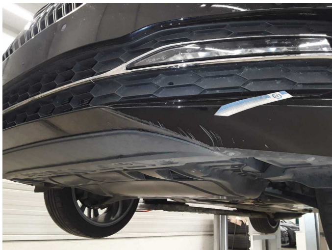
Damage 9: Front bumper: Front bumper - Scratched - Paint
