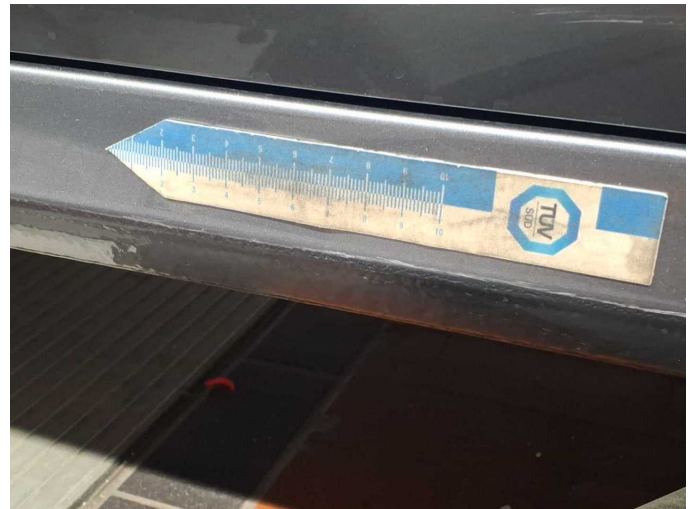
Damage 10: Sill - right side: Sill - Scratch(es) - Paint
