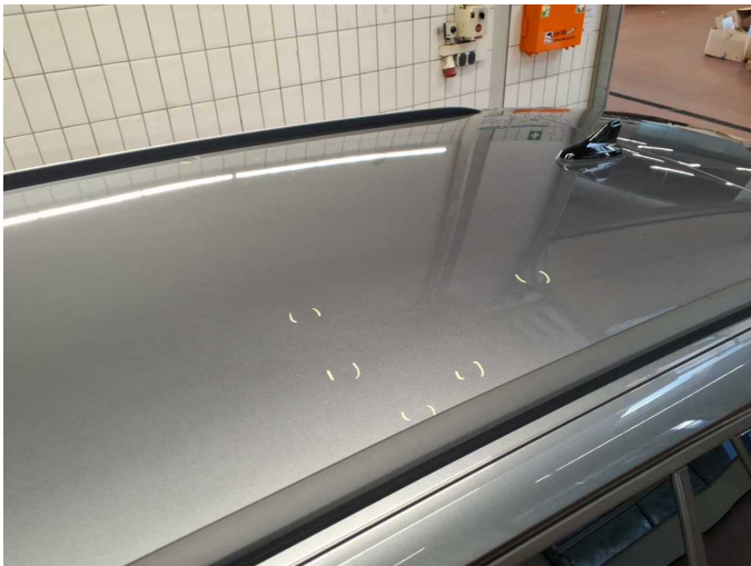
Damage 18: Roof: Roof (Verätzungen + ca 10 Dellen) - Dent / paintcoat damage - Repair and paint
