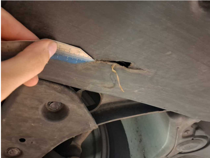
Damage 9: Body: Underbody panelling - Broken / torn - Replace
