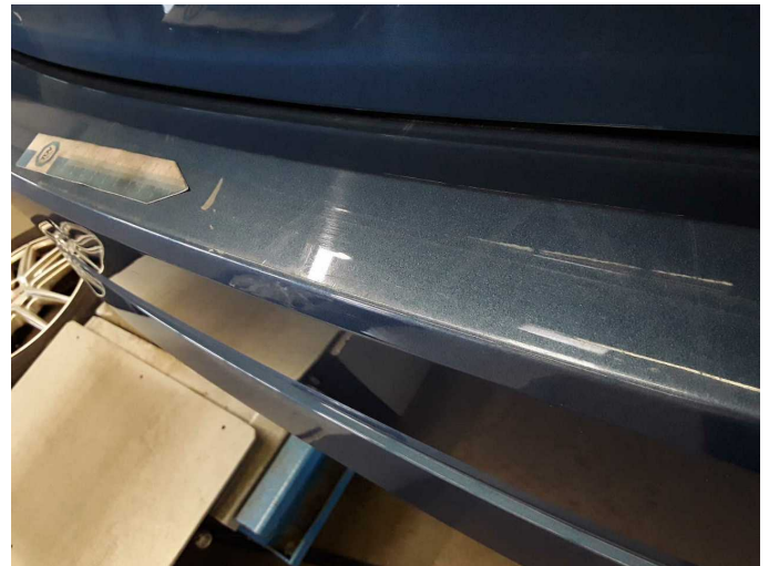
Damage 4: Rear bumper: Rear bumper - Scratched - Paint
