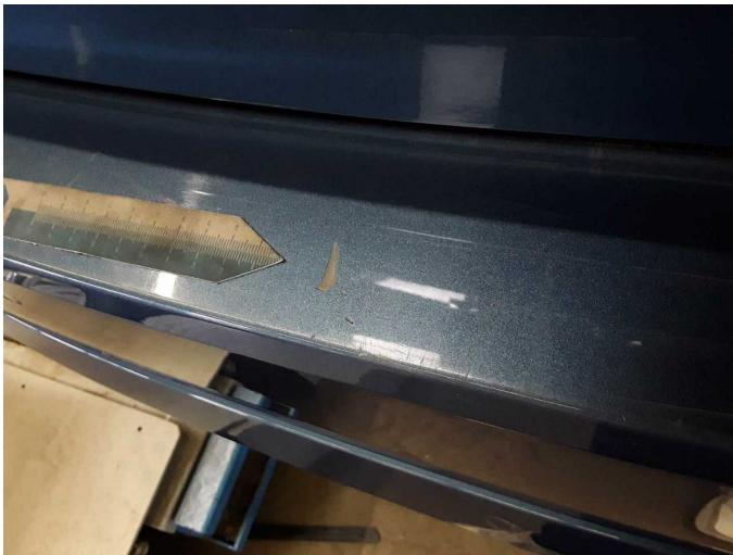
Damage 4: Rear bumper: Rear bumper - Scratched - Paint
