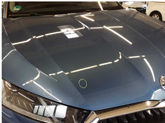
Damage 6: Bonnet: Bonnet - Corrosion - Repair and paint
