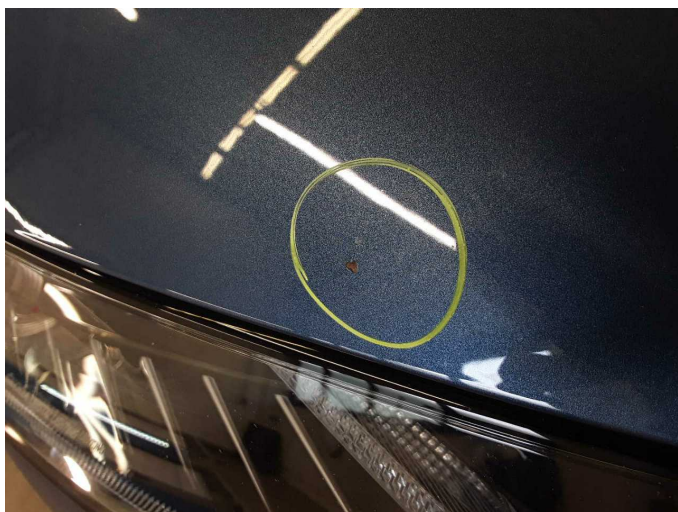
Damage 6: Bonnet: Bonnet - Corrosion - Repair and paint
