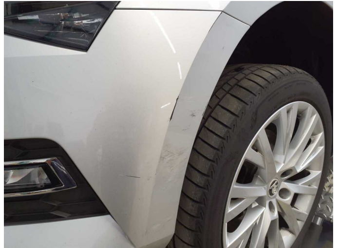
Damage 3: Front bumper: Front bumper - Scratched - Paint
