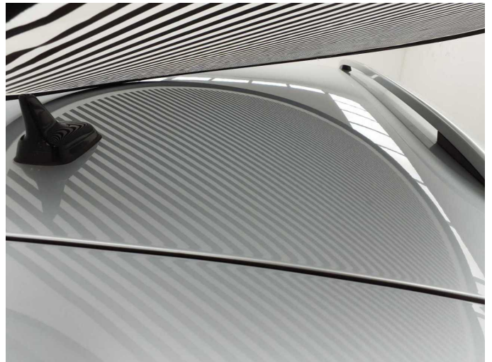
Damage 1: Roof: Roof (3x) - dent(s) - Smooth repair work
